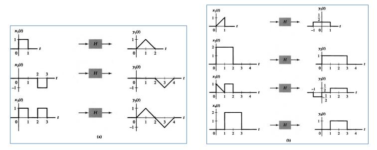
3<mark>. For a linear time invariant (LTI) system, if the output of the system y1(t) is known for a particular input x1(t) as shown below, compute the output of the same system for an input x(t) shown:</mark>
