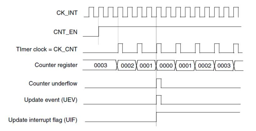
Counter timing diagram, Update event with ARPE=1 (counter underflow)
