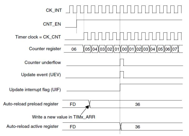
Counter timing diagram, Update event with ARPE=1 (counter overflow)
