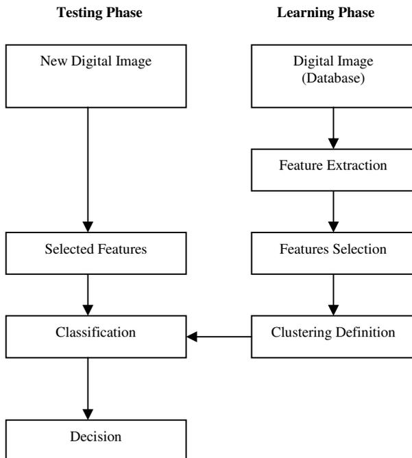
Fig. 2. Our system for mass detection in digitized mammograms.
