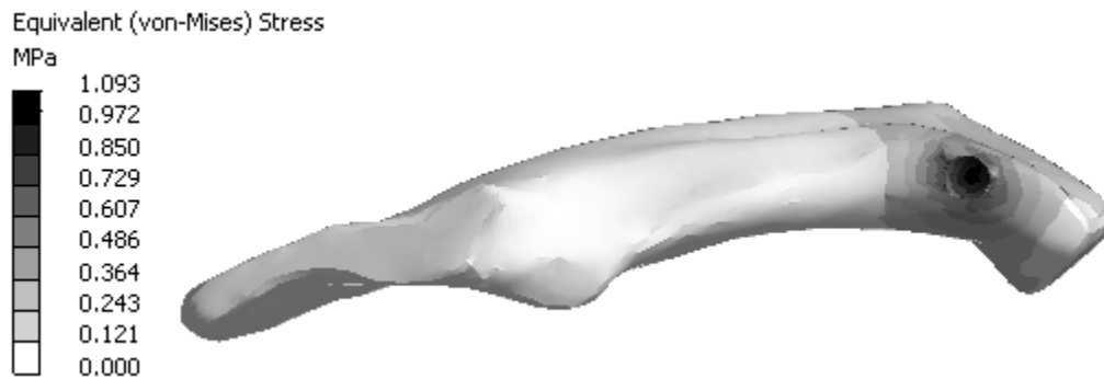
Fig.7. The von Mises stress distribution on the cancellous jaw bone at level 4 of the osseointegration process.
