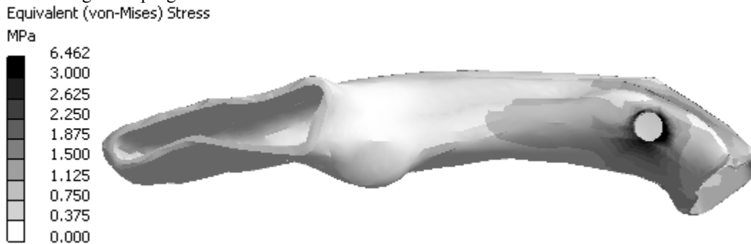
Fig. 5. The von Mises stress distribution in the cortical jaw bone at level 4 of the osseointegration.
