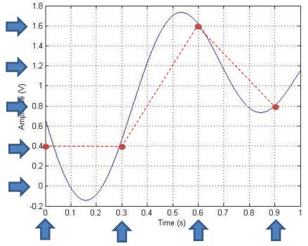
Comment: Digital signal does not represent original analog signal well. Reason: Insufficient sampling
