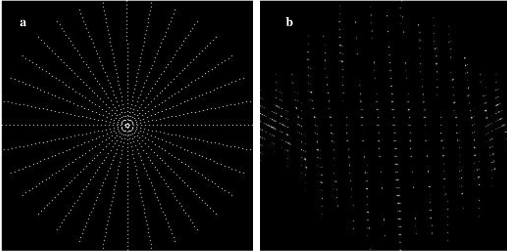
**Figure 1.** Illustration of the energy compacting transformation. (a) polar trajectory used and (b) the constructed system matrix after the energy compacting transformation with only a few nonzero elements.
