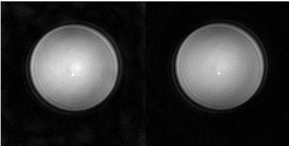
**Figure 2.** Images constructed with the new method (left) and the best image obtained with conventional gridding procedure (right).
