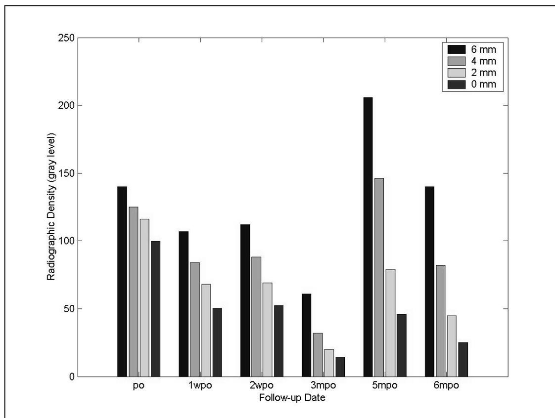
**Figure 3.** Measured calibration values from the step-wedge phantom (Aluminum thicknesses 2 to 6 mm) and the background of the x-ray image (assumed as the 0 mm Aluminum value). Notice the wide variations between different images from the same animal under different imaging and/or film development conditions.
