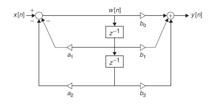
• Cascade Form:  $H(z) = \prod H_i(z)$  $H_1(z) H_2(z) H_N(z) y[n]$ *x*[*n*] —  $H_i(z)$  first- or second-order direct form II realization  $H(z) = \left[\frac{3(1+z^{-1})}{1+0.5z^{-1}}\right] \left[\frac{1+0.2z^{-1}}{1-0.4z^{-1}}\right]$ w[n]3 *v*[*n*] x[n]y[n]*z*<sup>-1</sup> *z*<sup>-1</sup> 0.5 3 -0.40.2
