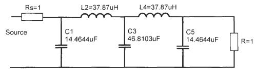
Convert the following normalized lowpass filter with into a bandstop filter with center frequency of 50 Hz and band of rejection from 45-55 Hz (3dB) assuming source/load resistance of 50Ω.
