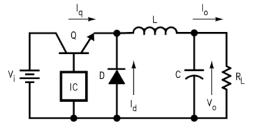
6. For the shown switching regulator, given that  $V_i$ = 5V that T= 10 µs and switch Q on time or  $t_{(on)}$ = 2µs. Draw the waveforms for  $V_o$  and  $I_g$  for one complete cycle.
