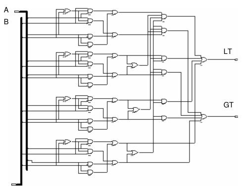
Schematic for a 4-bit magnitude comparator circuit
