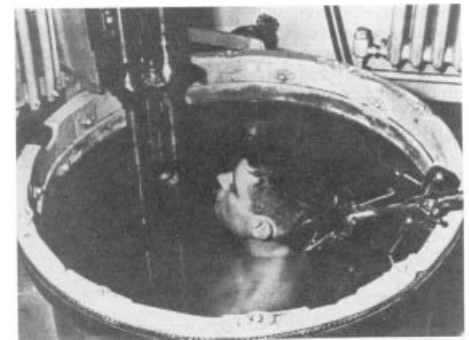
One of the first ultrasonic scanners for imaging the human body required that the patient be immersed in warm saline solution in a large metal tank in which a transducer rotated about the patient. Head scanning was not often performed with this technique. Shown here is the compound scanner (Somascope) developed by Howry and co-workers from a B-29 gun turret. (From Am. J. Digest Dis. 1963; 8:12. Harper and Row, Hoeber Medical Division. Used with permission.)
